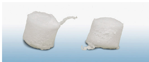
Coperion's new EGR knife minimises fine generation. Pellets produced on the new system (right) shown compared to current technology
