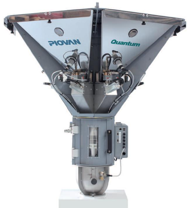
from the weighing pan to the mixer by the dump flapper, which opens and closes pneumatically. The mixer is spherical and the mixer blade is round to fit its geometry and prevent material stagnation problems. Its strength lies in an intelligent sensor that employs the surface of the mixer as a sensitive element, needing no adjustment caused by powder, electrostatic charges, or changes in material and blend density. The sensor is an integral part of the mixer's design.
